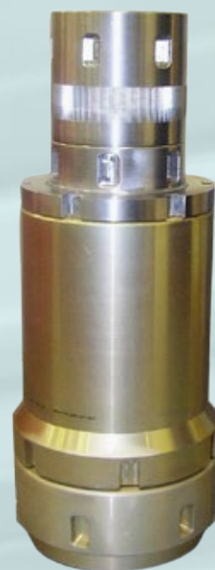
Special strain-relief backshell invented by Glenair for use on the French TGV rail system. This backshell design resolved complex intercar vibration and shock problems which resulted in destructive cable damage.
