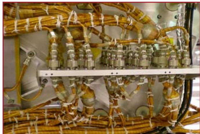
Subassembly-to-I/O-Panel level connectors and cables destined for extraterrestrial duty on Mars. The connectors shown are Glenair Series 80 "Mighty Mouse" which are specified for their reduced size and weight compared to standard Mil-Spec connector series.
