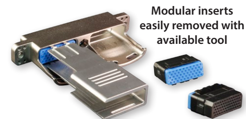
PATTERN 48 48 X Size 23 Contacts DWV= 1300 VAC DWV@50 000 ft = 800 VAC
