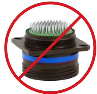
Non-parylene-compatible PCB connector. Resilient rubber seal is wholly inadequate to the task of sealing internal / conductive connector components during parylene vacuum deposition process.
