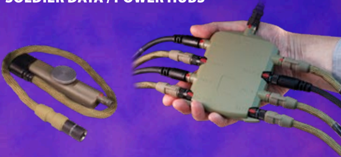
STAR-PAN™ Integrated soldier multiport USB data hub / power distribution systems
