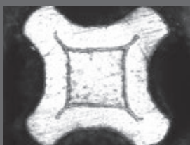
Transverse cross-section of a TwistPin contact crimp, solid wire
