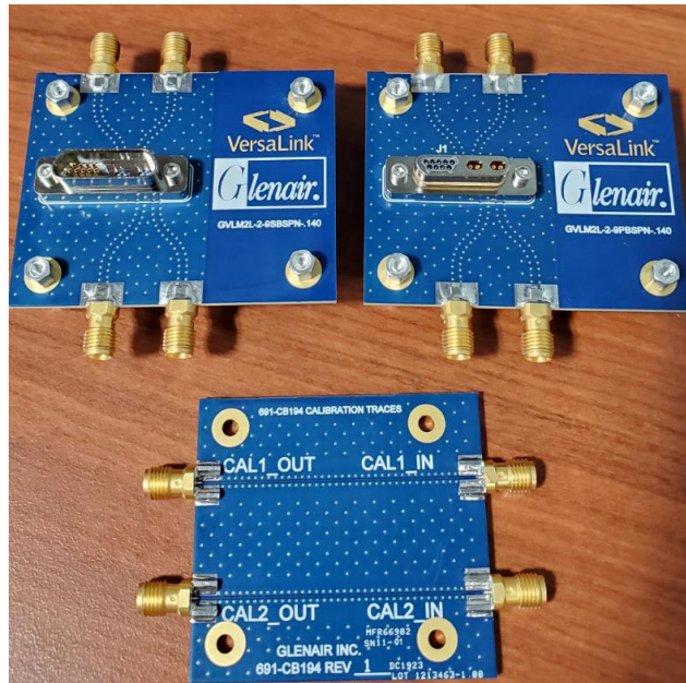
Figure 1. Straight Micro-D test fixtures and 2x-trace calibration PCB
