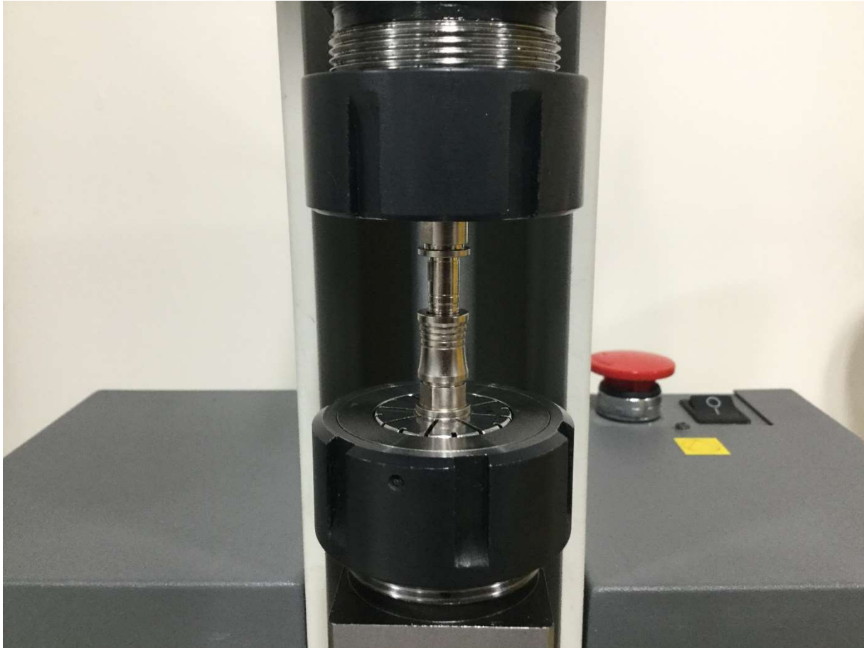
Figure 7: Mating Durability Test Setup (Detailed View)
