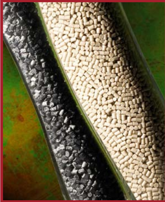
Glass-filled composite thermoplastic resins in pellet form, ready for use in injection molding applications.
