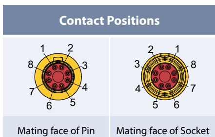
El Ochito® Red for Multi-Gigabit 100 Ohm Datalinks, pin contact mating face
