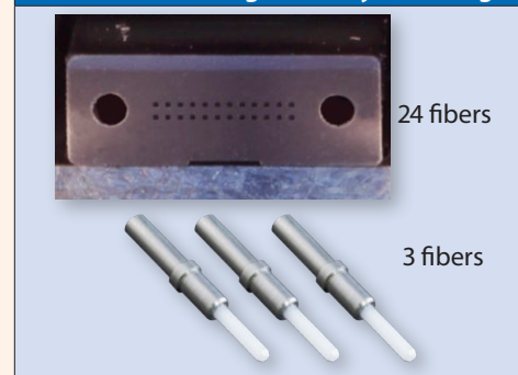
Up to 24 fibers in a single compact, lightweight ferrule (7mm x 3mm / .276" x .118")—same real estate as three size #16 termini side by side
