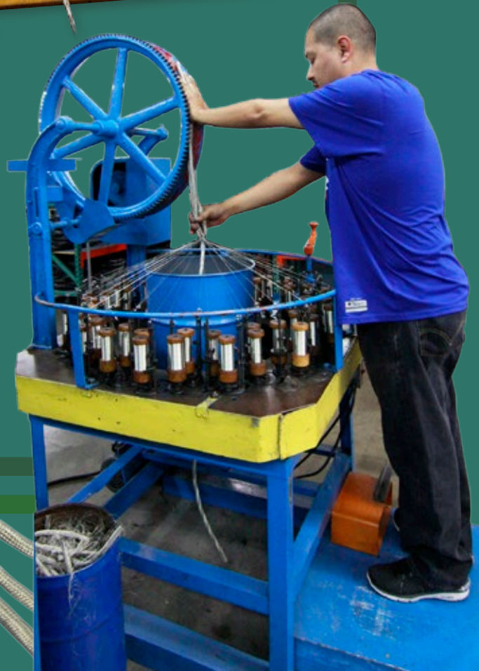
▶ Complete coverage of cable interstices in overbraided assemblies
